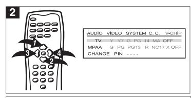
Press the Navigation  ${}^{}_{\bullet}$  or  ${}^{}_{\bullet}$  **@** button to select the TV rating, then press the Navigation  ${}^{}_{\leftarrow}$  **@** or  ${}^{}_{\rightleftharpoons}$  **@** button to set the TV rating.
