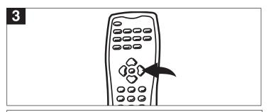
When CH. SEARCH is selected, press the Navigation ⇒ button to start the Auto Search. The TV will automatically cycle through all the channels and store active channels into memory. When completed, the TV will be on the first available channel.
