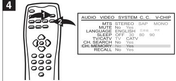
Using the Navigation  $\Leftrightarrow$  **0** or  $\Rightarrow$  **2** button, select NO to skip the channel or YES to keep the channel.
