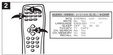
Select a channel to be skipped or added using the CHANNEL Up 1 or Down 2 button.
