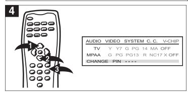
Press the Navigation  ${}^{}_{\bullet}$   ${}^{}_{\bullet}$  or  ${}^{}_{\bullet}$   ${}^{}_{\bullet}$  button to select CHANGE PIN, then enter the desired pin number using the Direct Channel Selection buttons  ${}^{}_{\bullet}$ ; then confirm again using the Direct Channel Selection buttons  ${}^{}_{\bullet}$ .
