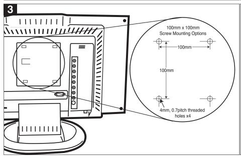
This monitor conforms to the VESA Flat Panel Mounting Physical Mounting Interface Standard which defines a physical mounting interface for flat panel monitors, and corresponding standards for flat panel monitor mounting devices, such as wall and table arms. The VESA mounting interface is located on the back of your monitor. The VESA Mounting slots of this model are located inside the handle cover (shown in the following figure).
