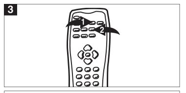
Adjust the volume level by pressing the VOLUME Up ① or Down ② button. The volume level will be indicated on the screen by green bands and a green numerical display between 0 and 24 where 0 is the lowest setting and 24 is the loudest.
