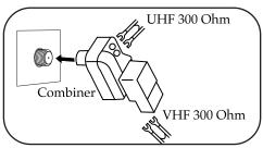
Connect the UHF twin-lead wire to a combiner (NOT SUPPLIED). Connect the VHF twin-lead to a 300-75 ohm matching transformer (NOT SUPPLIED). Attach the transformer to the combiner. Attach the combiner to the antenna jack.
