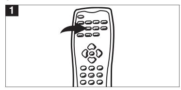
Press repeatedly to set the sleep time between "10" and "90" (each press will increase the time by 10 minutes). When the sleep time is up, the TV will shut off.
