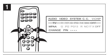
Enter the TV menu, then select V-CHIP using the Navigation  $\Leftrightarrow$   $\bullet$  or  $\Leftrightarrow$   $\bullet$  button. Press the Navigation  $\diamondsuit$  button  $\bullet$ , then enter the pin number using the Direct Channel Selection buttons  $\bullet$ . When first using the unit, the pin number is set to "1234".
