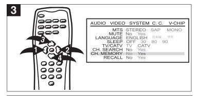
Select the SYSTEM menu using the Navigation ← ● or ⇒ ● button. Use the Navigation ↑ ● or ∜ ● button to select CH. MEMORY.
