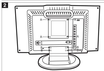
Remove the four (4) screws (A) using a phillips head screwdriver and remove the handle.
