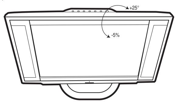
To adjust the base so it is at 90°, simply press the Release button on the bottom of the stand. This is useful for storing the monitor.
