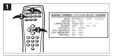
Press the POWER button ● to turn on the TV; the POWER indicator will light green. Press the TV/AV/PC button ❷ until TV or CATV appears. Select the TV or CATV option as described on page 17. Press the ▶ button ❸; the MENU screen will appear
