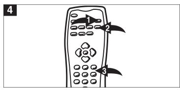
For proper operation, before selecting channels, they must be set into the TV's program memory, see page 22. Press and release the CHANNEL Up ① or Down ② button. The TV automatically stops at the next channel set into memory. This will not operate if channels are not set into memory.
