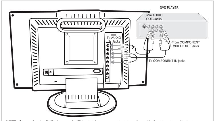
**NOTE:** Connecting the DVD player to the TV using the component cables will provide the highest quality picture. Connecting using an S-video cable will provide the next highest quality picture, followed by standard Audio/Video cable connection.
