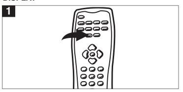
Press the DISPLAY button once to show the mode (i.e. S-VIDEO) and audio mode. Press again to clear the display.
