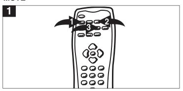
Press the MUTE button • to turn off the sound. The TV's sound will be silenced and "MUTE" will appear on the screen. The sound can be turned back on by pressing this button again or the VOLUME Up • or Down • button.
