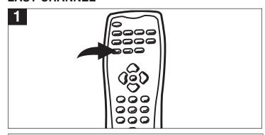
Press the LAST CH button to go back to the last channel selected. Press the LAST CH button again to return to the channel you were watching.
